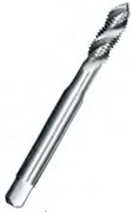
DIN 371/C 35° HSS M2 (standard) M35 (cobalt) 63-64 HRC R<750 N/mm 2 (standard) R<850 N/mm 2 (cobalt)
