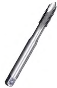
DIN 371/B HSS M2 (standard) M35 (cobalt) 63-64 HRC R<750 N/mmq (standard) R<850 N/mmq (cobalt)
