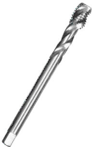
DIN 376/C 35° HSS M2 (standard) M35 (cobalt) 63-64 HRC R<750 N/mm 2 (standard) R<850 N/mm 2 (cobalt)
