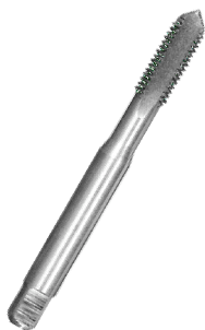
DIN 371/C HSS M2 (standard) M35 (cobalt) 63-64 HRC R<750 N/mm 2 (standard) R<850 N/mm 2 (cobalt)
